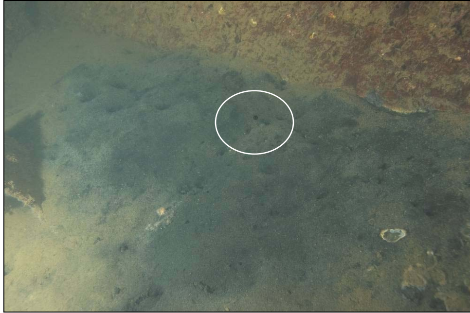
Figure 9.25. Sediments in crew’s galley area forward of Memorial. Dark areas are oil saturated sediments. White oval circles a drop of released oil moving toward the surface (NPS Photo by Brett Seymour).
