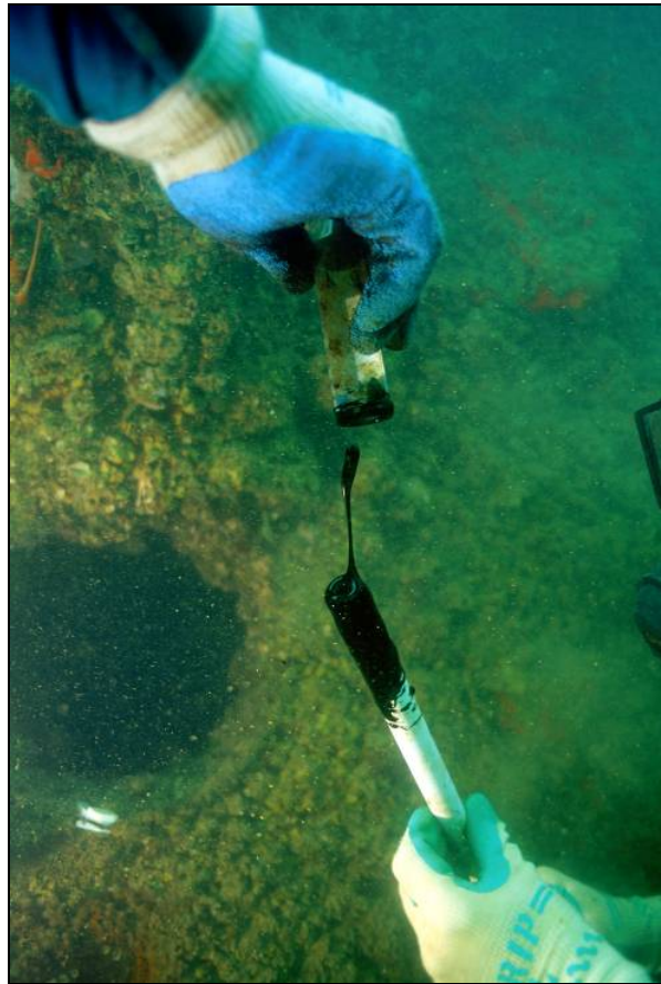
Figure 9.18. Internal oil measurement and oil sample collected by reaching PVC pipe in porthole and pushing vertically to the overhead. Overhead oil depth is indicated by oil on pipe (NPS Photo by Brett Seymour).
