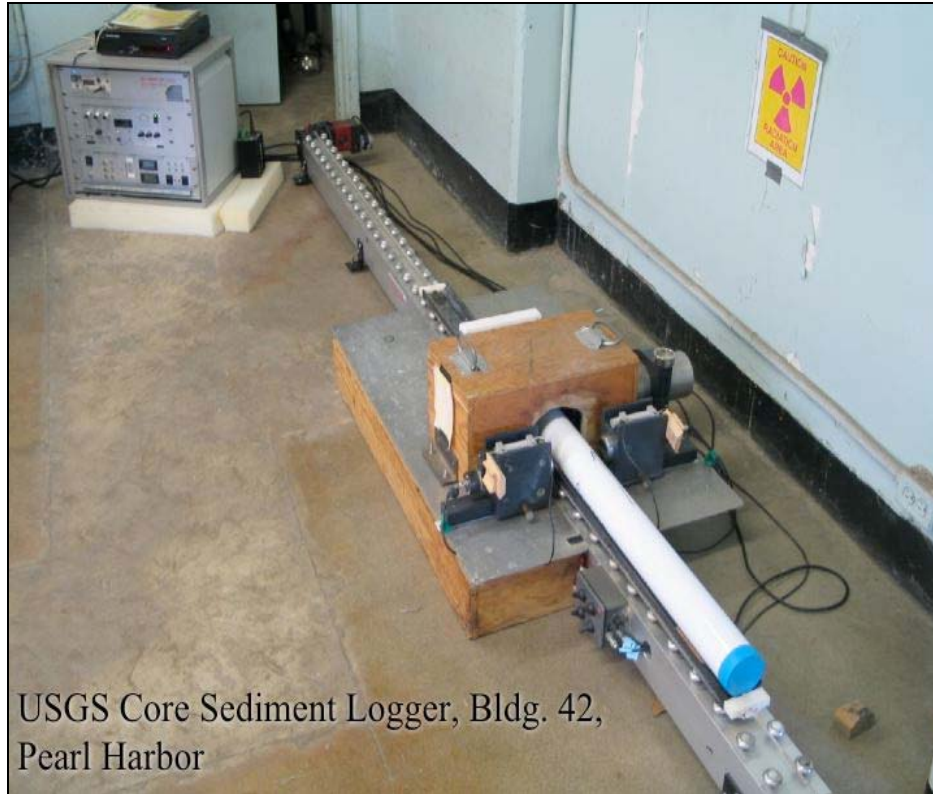
Figure 10.10. USGS core sediment logger set up in Navy Building 42 during the drilling operations. An enameled steel Shelby tube is being scanned (USGS Photo).
