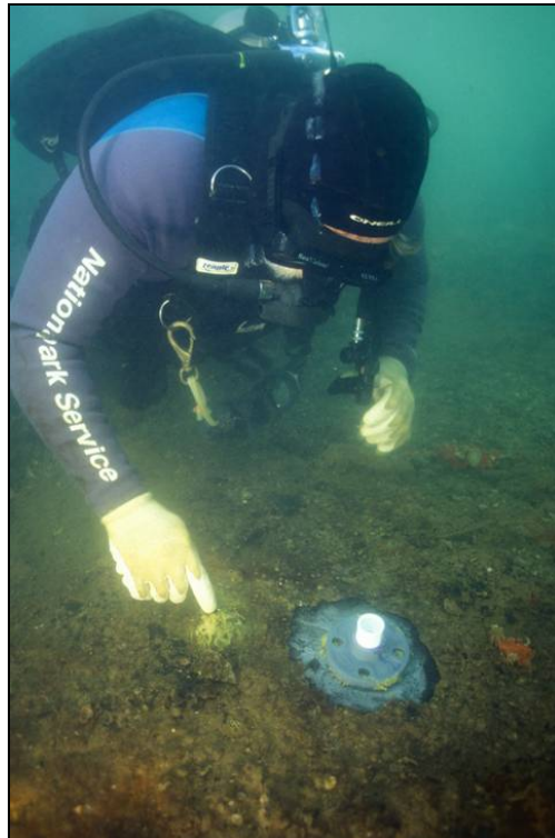
Figure 9.5. Comparison of the original, left, and current GPS monitoring points. Note: 2001 epoxy covered by pioneering organisms (NPS Photo by Brett Seymour).
