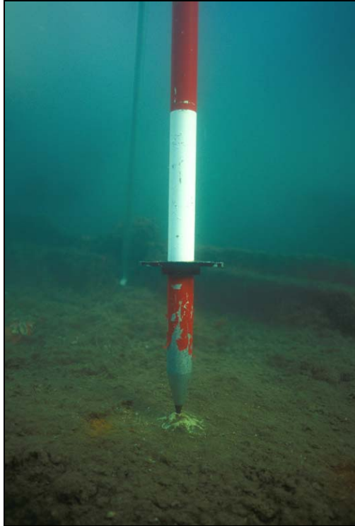
Figure 9.4. Surveying GPS monitoring points on Arizona , here using original velocity tool-set, stainless steel bolt surrounded by epoxy (NPS Photo by Brett Seymour).
