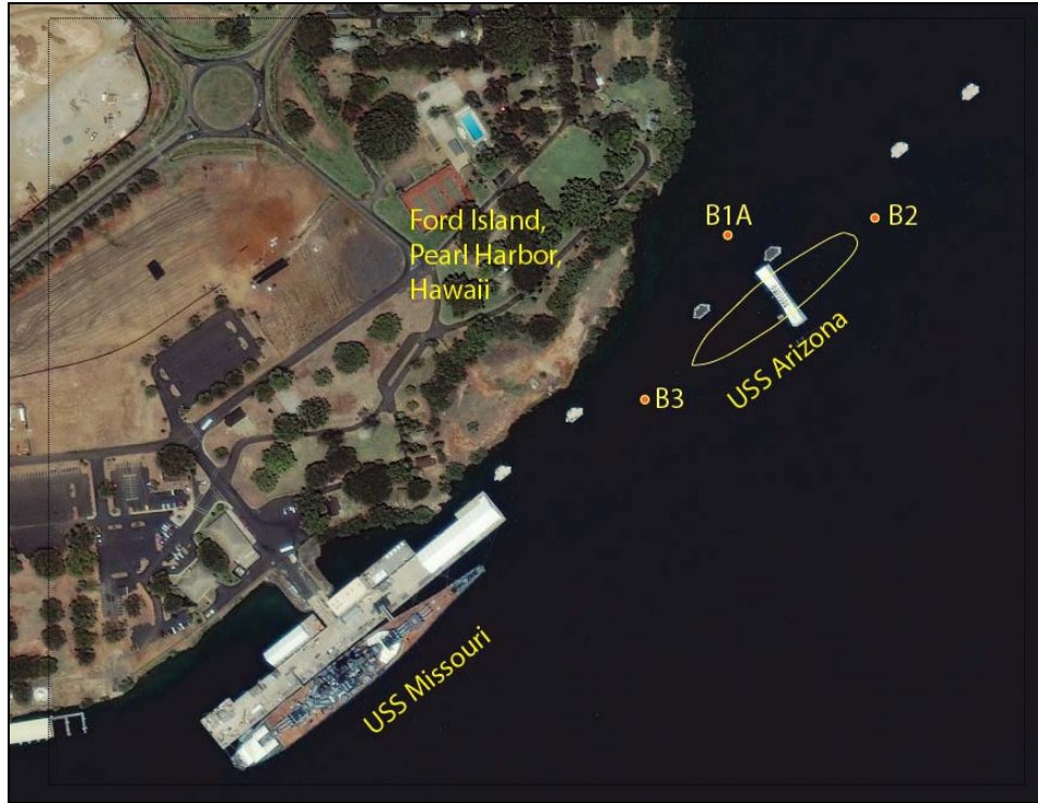
Figure 10.1. Boreholes B1a, B2 and B3 located around the hull of USS Arizona, west of Ford Island.
