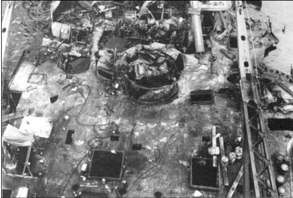
Figure 10.5. Salvage crews in 1942 were able to work on the deck above water and cut entry-ways into the vessel for recovery operations (USS Arizona Memorial Photo Archive).
